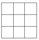
If we replace each pixel by a weighted average of its neighbourhood pixels then the response of the linear mask for the pixel  $z_5$  is  $\sum_{i=1}^{9} w_i z_i$ . We may repeat the same process for the whole image.
