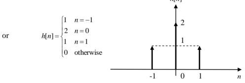
The above response applied to a signal x[n] yields a signal y[n] = x[n-1] + 2x[n] + x[n+1] or in z-transform domain  $Y(z) = (z^{-1} + 2 + z)X(z) \Rightarrow Y(j\omega) = 2(\cos \omega + 1)X(j\omega)$ . Therefore,
