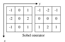
If we consider the left mask of the Sobel operator, this causes differentiation along the y
